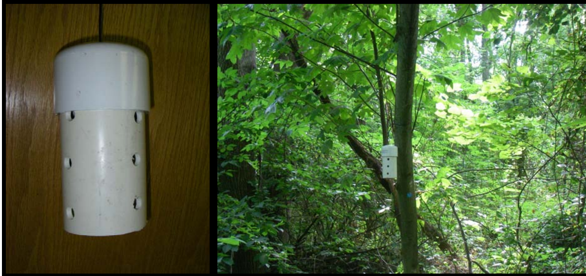
Figure 2. PVC shield for air temperature HOBO. Dimensions: 3in PVC, 6in long, 1/2in drilled holes for air flow (12)
